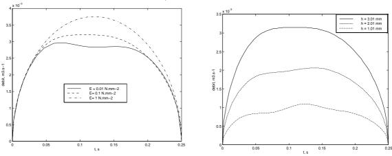
Figure 5: Simulated limitation of the volume flow velocity: influence of the velum stiffness (left) and the constriction size (right).
