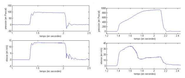
Figure 7: Pressure drop (top) and volume flow velocity (down) measured for two conditions: *Left*: low pressure drop; normal conditions *Right*: high pressure drop; pathological conditions with sleep hypopnea.
