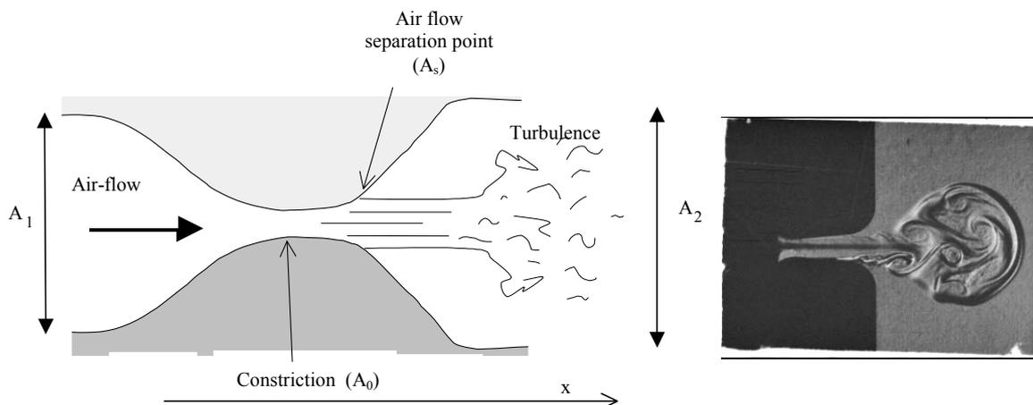
Fig. 3: Schematic Illustration for airflow inside the constriction.
