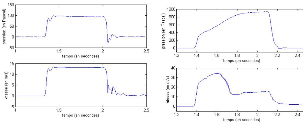
Figure 7: Pressure drop (top) and volume flow velocity (down) measured for two conditions:
