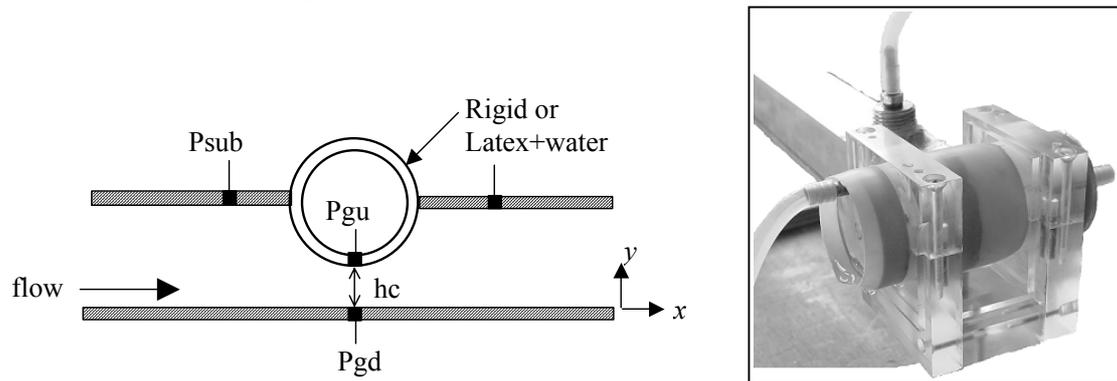
Figure 6: Schematic view and photography of the experimental setup used to study airflow/tongue interaction.
