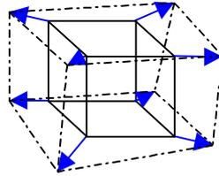
**Fig. 2. Applying a trilinear transformation to a cube**
