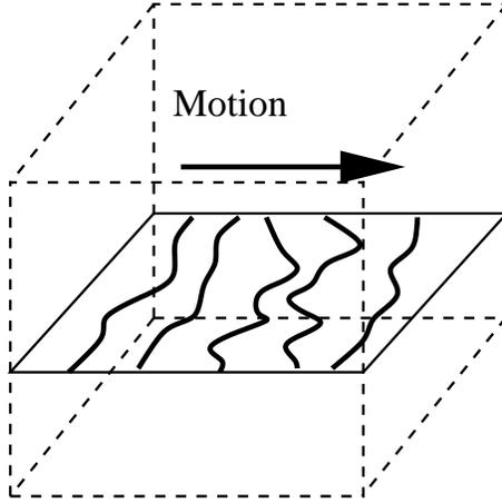
Figure 1: Dislocations in a slip plane f homo
