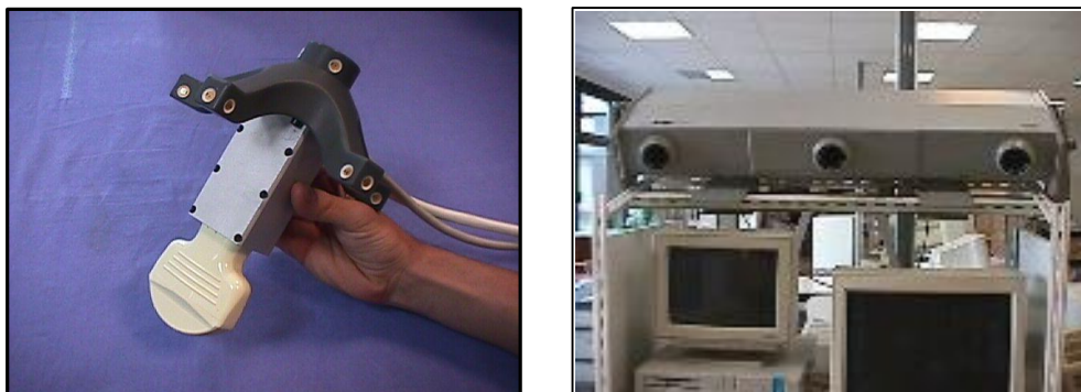
Figure 1: Echographic set-up: (left) the echographic probe equipped with infrared diodes - (right) the three cameras for diodes localization and tracking and position measurement.
