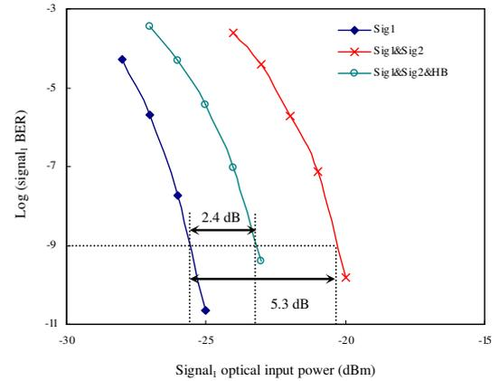
Fig. 5: BER of signal<sub>1</sub> vs. its optical input power for signal<sub>1</sub> (1535 nm) in three cases: alone (Sig1), with signal<sub>2</sub> (Sig1&Sig2) and with signal<sub>2</sub> and the HB at the transparency wavelength (Sig1&Sig2&HB). The SOA drive current is 120 mA.
