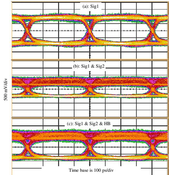
Fig. 6: SOA output eye diagrams of signal<sub>1</sub> in three situations: (a) alone (Sig1), (b) with signal<sub>2</sub> (Sig1&Sig2) and (c) with signal<sub>2</sub> and the HB at the transparency (Sig1&Sig2&HB). The optical input average power of signal<sub>1</sub> (1535 nm) is about -15 dBm and that for signal<sub>2</sub> (1560 nm) is around -7.5 dBm. The SOA bias current is 120 mA.
