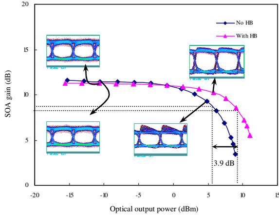
Fig. 4: SOA saturation curves of signal<sub>1</sub> and its optical eye diagrams obtained in dynamic regime, in presence and in absence of the HB. The SOA drive current is 120 mA.
