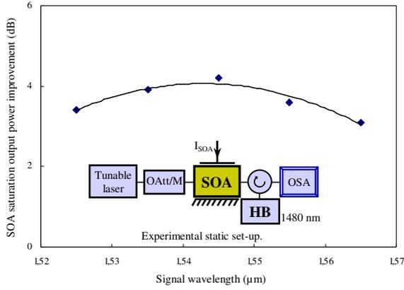
Fig. 1: SOA 3-dB saturation output power enhancement, due to the HB employment, dependency on input signal wavelength. Points present measurements and solid lines present polynomial approximation. (OAtt/M: Optical attenuator/monitor and OSC: Oscilloscope).
