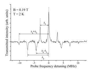
FIG. 7: Hole-burning transmission spectrum for Tm<sup>3+</sup>: YAG under a 0.19 T magnetic field. The spectral holes and antiholes correspond to site 3 and 5 ions. The features corresponding to site 1 are out of the probing spectral window.
