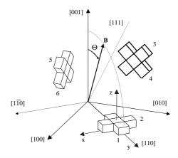
FIG. 3: Tm substitution sites in the YAG matrix. In each site, the transition dipole moment  $\vec{\mu}$  is represented by an oblong and is directed along the local Oy axis. Here the local frame x,y,z is given for site 1. The direction of the magnetic field **B** is defined by angle  $\Theta$ .
