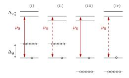
FIG. 6: (color online) Optical pumping of four classes of ions to the non-resonant ground sublevel by excitation at frequency  $\nu_0$ . Solid lines: strong transitions. Dashed lines: weak transitions. Ions are depicted by open circles.
