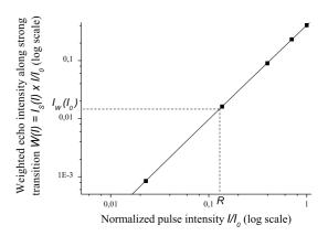
FIG. 13: Weighted echo intensity on the strong transition for different excitation pulse intensities (squares). Theses values are interpolated with a straight line (solid line) in order to solve Eq. 17. A graphical solution is given by the intersection point of  $W(\mathcal{I}) = \mathcal{I}_s(\mathcal{I}) \times \mathcal{I}/\mathcal{I}_0$  and  $W(\mathcal{I}) = \mathcal{I}_w(\mathcal{I}_0)$ . The value is directly read out as  $R = \mathcal{I}/\mathcal{I}_0$  at the intersection.
