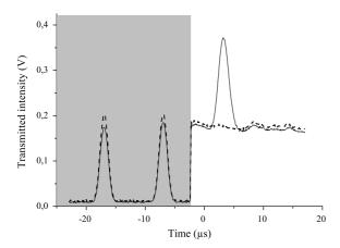
FIG. 12: Photon echo in  $Tm^{3+}$ : YAG under magnetic field with two gaussian pulses at T=2.6 K (solid line) and T=1.9 K (dashed line). The detection channel is gated by an acousto-optic modulator (AO 3 in Fig. 5) which attenuates the excitation pulses (grey area). This AOM opens a few  $\mu$ s after the second pulse to let the photon echo through. The echo disappears when optical pumping dominates thermalization.
