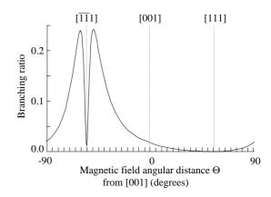
FIG. 4: Theoretical branching ratio variations for ions in sites 3 and 5 as a function of magnetic field orientation<sup>24</sup>.
