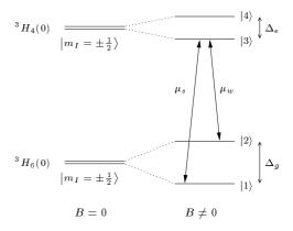
${\it FIG.}$  2: Building a three-level system with nuclear spin levels in thulium.
