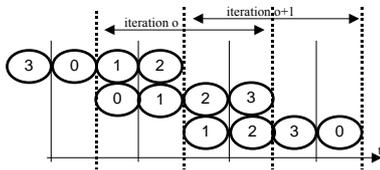
Figure 9: Pipelined architecture
