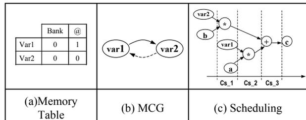
Fig. 3: Scheduling under I/O timing and latency constraint
