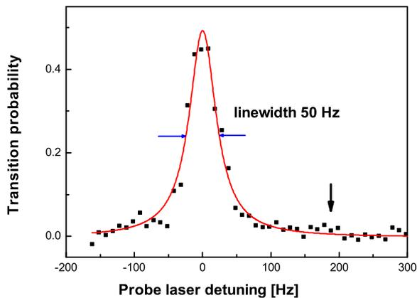
FIG. 2: Atomic carrier resonance at 698 nm for a probe time of 15 ms, a power of  $3 \mu\text{W}$  and lattice depth  $U_0 = 170 E_r$ . The vertical arrow is at a detuning corresponding to the transverse oscillation frequency for this value of  $U_0$ :  $\nu_{\perp} = 186 \text{ Hz}$ .
