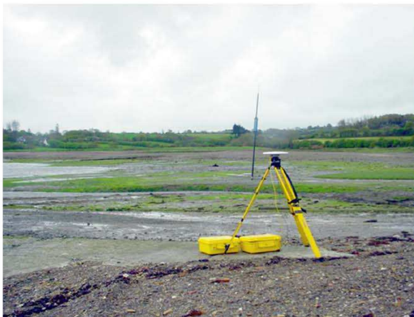
DGPS Trimble 5700 - station base
