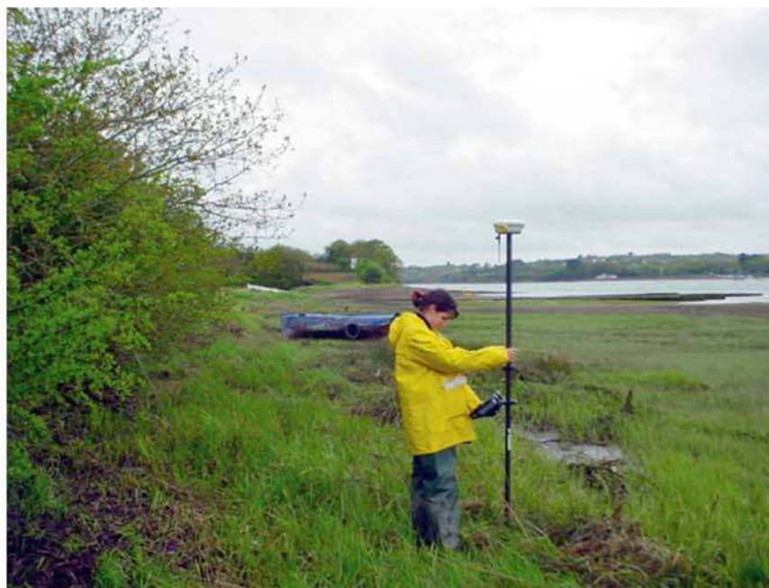
Mobile Trimble 5800 - station mobile
