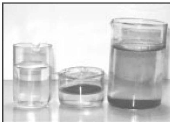
**Figure 3** From left to right: pure water, TC1 soot in water, and engine soot in water
