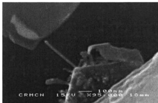
FIG. 11. Si NW linked at one extremity to a silicon bump deposited on the edge of a silicon step. Its other extremity is directed to the following silicon bump. Experimental conditions: laser power of 0.18 W, silane pressure of 5 mbars, and laser scan speed of 1 \mu\text{m/s} .
