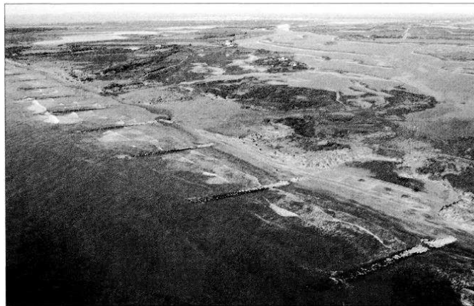
Photo 5 – Groyne field on the littoral of Petite Camargue (from Service Maritime et de Navigation du Languedoc-Roussillon, 1998).
