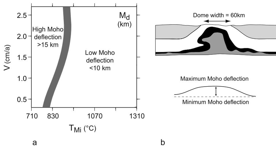
**Figure 8.** Moho deflection ( $M_d$ ) as a function of boundary velocity ( $V$ ) and initial Moho temperature ( $T_{Mi}$ ) for a 60 km wide dome. (a) Diagram showing the domains of low (<10 km) and high (>15 km) Moho deflection. The domain of low Moho deflection can be considered a mapping of the  $V$  and  $T_{Mi}$  conditions that favor the development of MCCs. (b) Sketch showing how the Moho deflection is measured.
