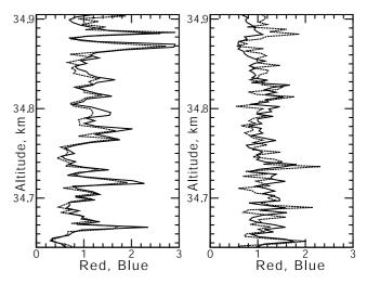
**Figure 2.** Comparison of two records of two-wavelength scintillations ((left) vertical V5, (right) oblique O6). Abscissa is red (dashed line) and blue (solid line) intensities normalized on the corresponding mean. Ordinates are altitude of ray perigee. The altitude of the curve for blue photometer was shifted 5 m downward in order to compensate for the calculated chromatic shift  $\Delta_{BR}$ .
