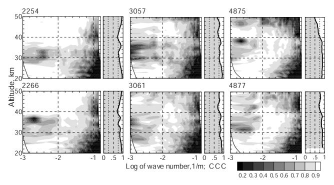
**Figure 3.** Close to vertical star set observations V1-V6. Estimates of coherency  $Coh_{i,j}$  (columns 1, 3, and 5) and correlation coefficients CCC (columns 2, 4, and 6). Orbit number appears above each plot. See color version of this figure at back of this issue.
