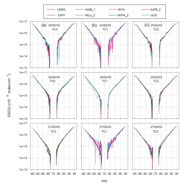
**Figure 6.**  $NO_2$  DSCDs measured by all groups on February 26, 27, and 28 for (a) TC0, (b) TC1, and (c) TC2 settings. The color code is also given on the figure.
