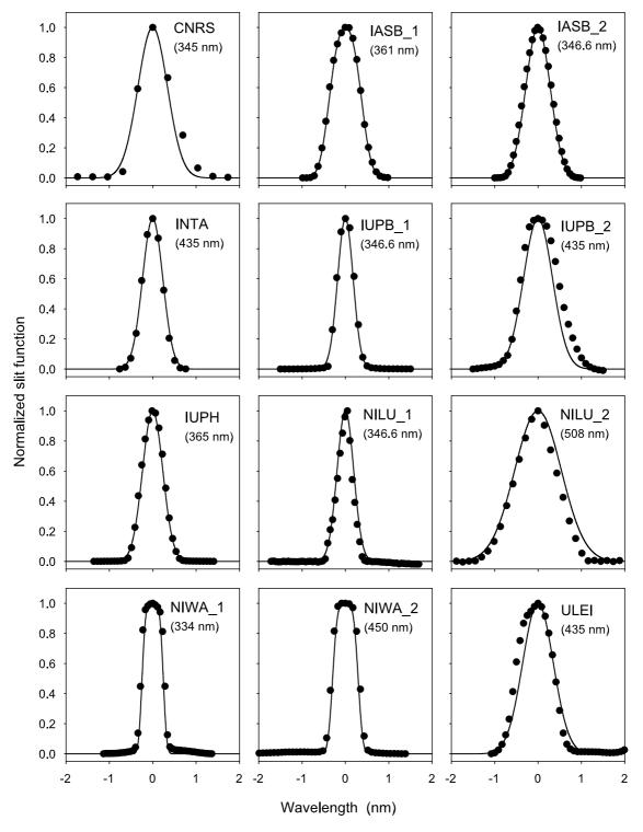
**Figure 3.** Slit functions of all participating instruments. Measured functions using a Hg lamp are represented by dots, while solid lines show the functions derived from zenith sky spectra using the WINDOAS program.
