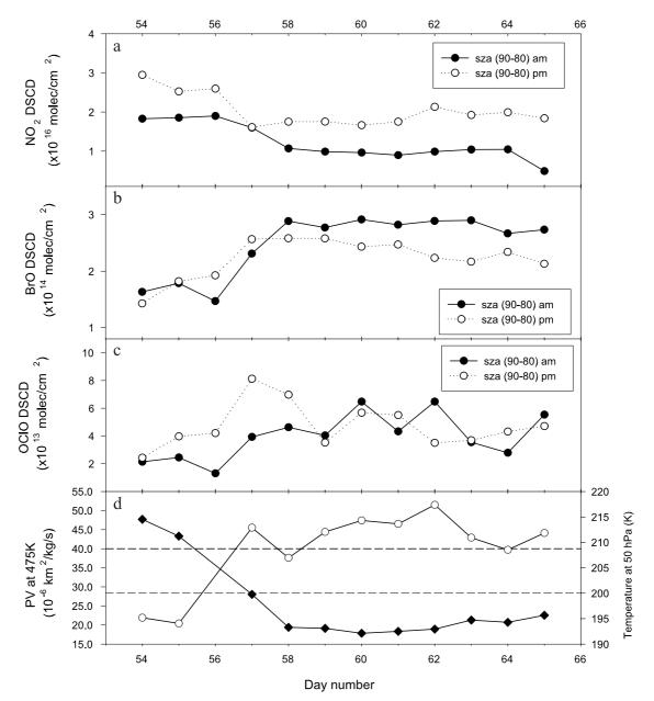
**Figure 2.** Evolution of the three target species during the campaign. (a) NO<sub>2</sub> DSCD at  $90^{\circ}-80^{\circ}$  sza am and pm. (b) BrO DSCD at  $90^{\circ}-80^{\circ}$  sza am and pm. (c) OCIO DSCD at  $90^{\circ}-80^{\circ}$  sza am and pm. (d) Potential vorticty (PV) at the 475 K isentropic level (open circles) and ECMWF temperature at 12 UT at 50 hPa (solid diamonds).
