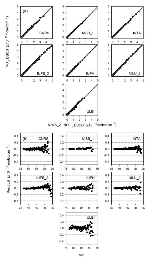
**Figure 5.** Illustration of the procedure used for selecting the  $NO_2$  reference groups (TC0, day = March 1). (a) Regressions between measurements of each instrument and those of NIWA\_2. The dashed line shows slope 1 and zero intercept. (b) Sza variations of residuals.
