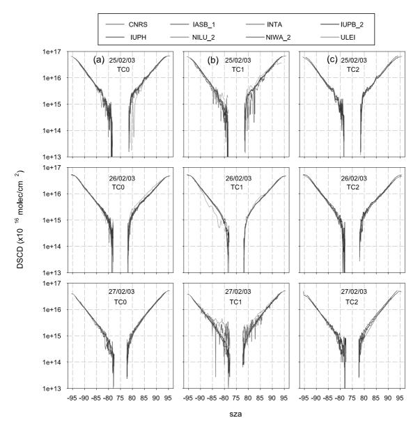
**Figure 6.**  $NO_2$  DSCDs measured by all groups on February 26, 27, and 28 for (a) TC0, (b) TC1, and (c) TC2 settings. The color code is also given on the figure. See color version of this figure at back of this issue.
