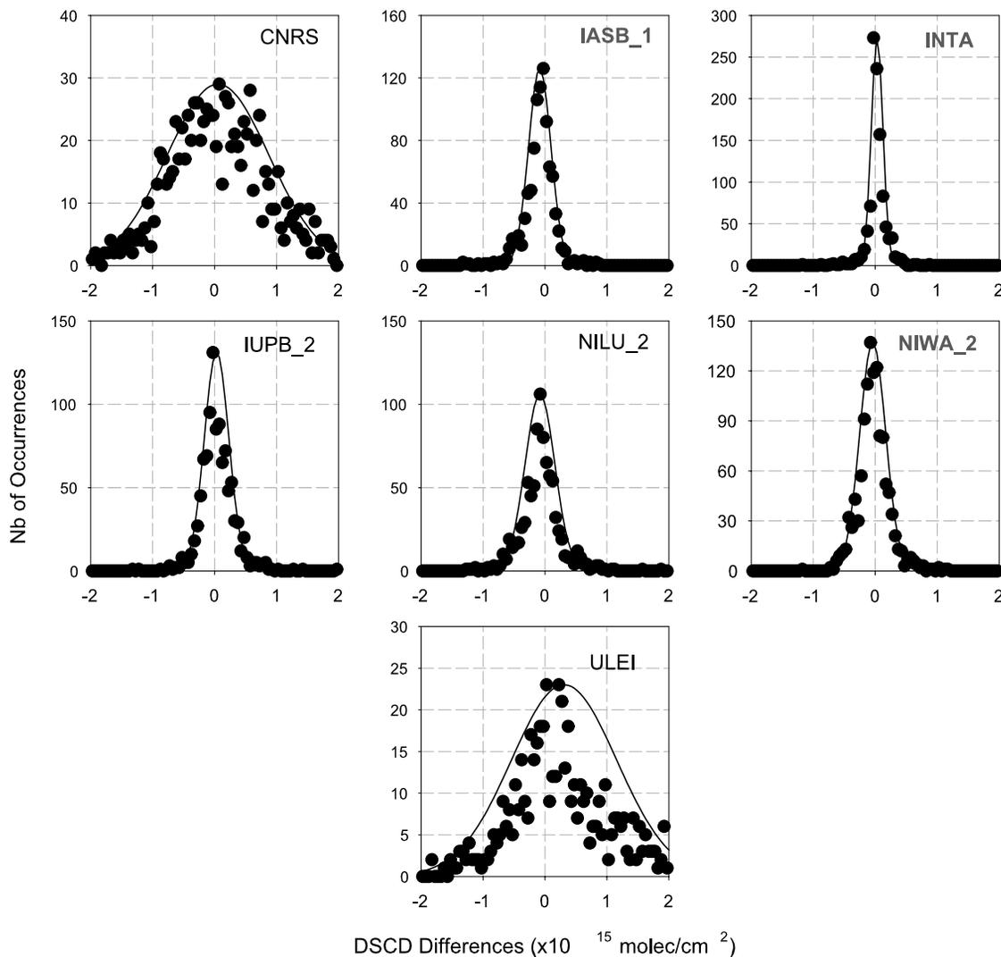
**Figure 10.** Histograms of DSCD differences for each instrument compared to the reference for TC1. The abscissa are the absolute differences observed between one instrument and the references, and the y-axis represent the number of occurrences of one specific difference value. The solid line shows the normal function of the same mean and standard deviation as the data.
