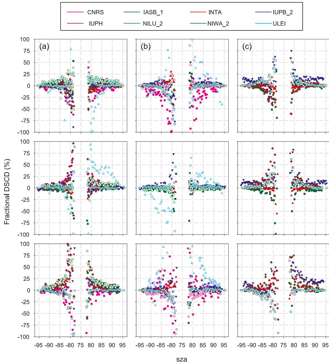
**Figure 7.**  $\text{NO}_2$  fractional differences for all groups on February 26, 27, and 28 for (a) TC0, (b) TC1, and (c) TC2 settings (solid circles, CNRS; solid squares, IASB\_1; solid triangles, INTA; solid inverted triangles, IUPB\_2; solid diamonds, IUPH; open circles, NILU\_2; open squares, NIWA\_2; open triangles, ULEI).
