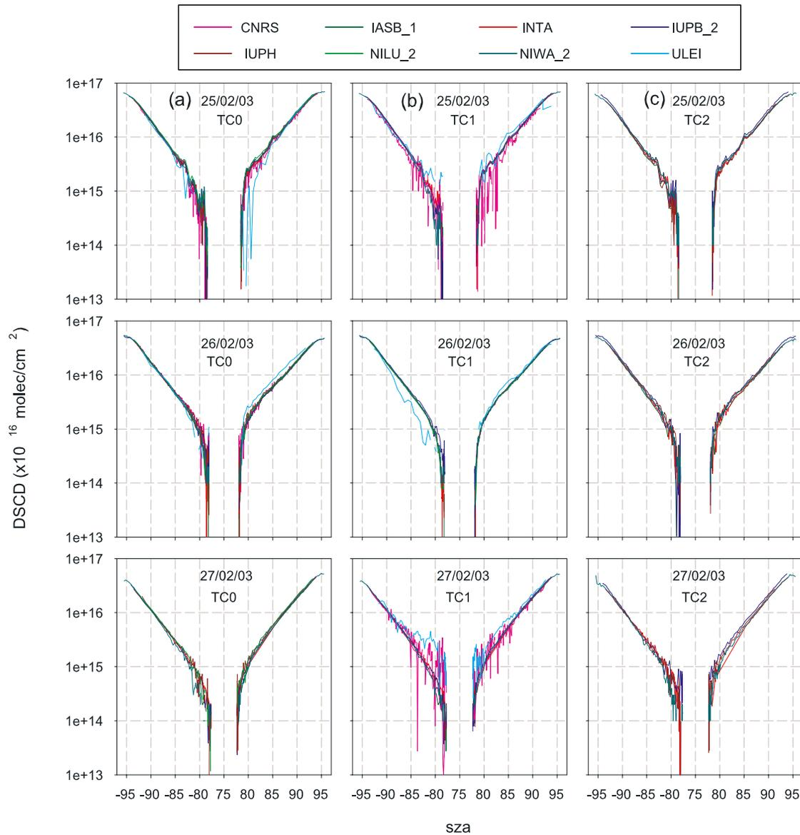
**Figure 6.** NO<sub>2</sub> DSCDs measured by all groups on February 26, 27, and 28 for (a) TC0, (b) TC1, and (c) TC2 settings. The color code is also given on the figure.
