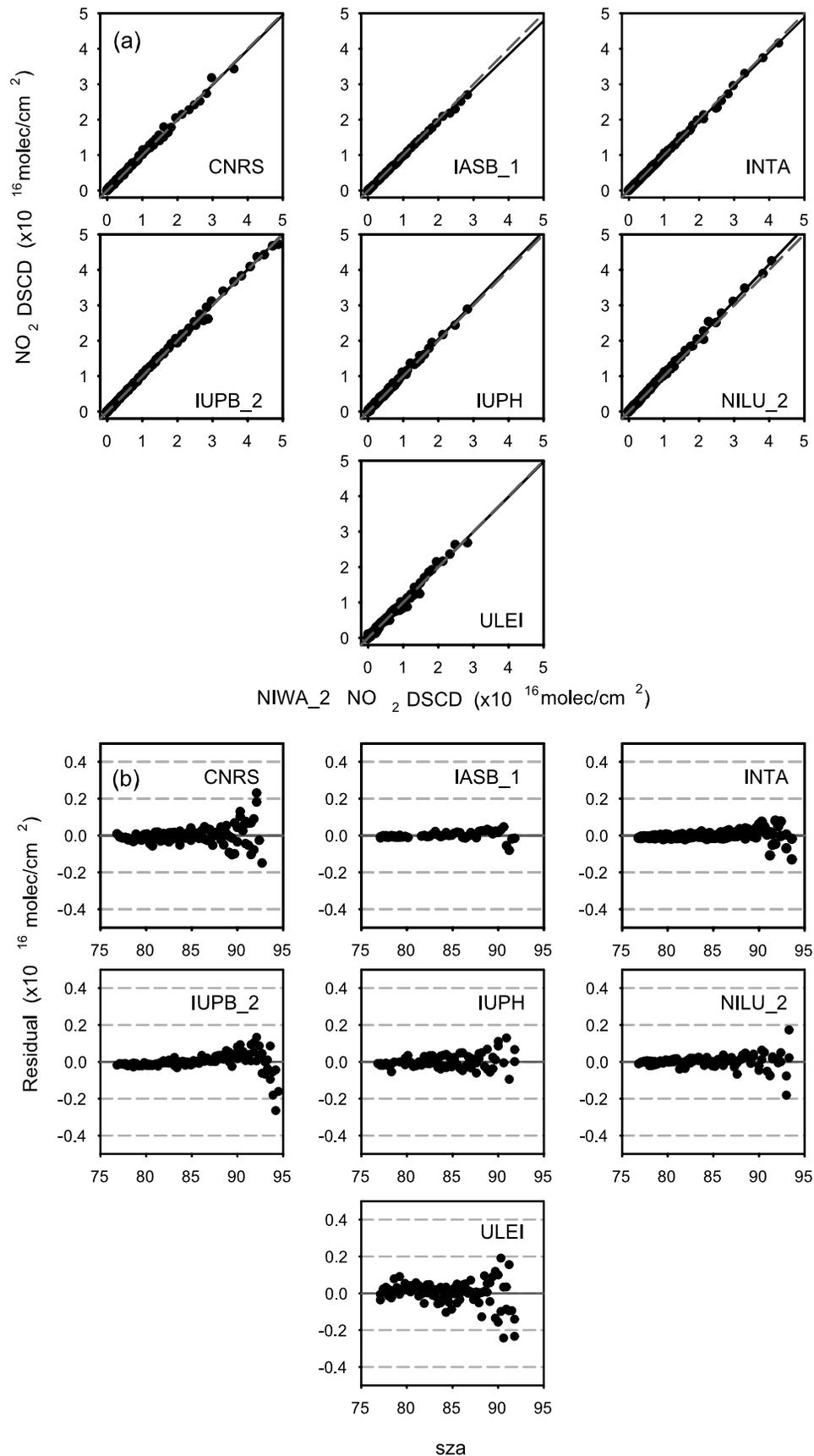
**Figure 5.** Illustration of the procedure used for selecting the  $\text{NO}_2$  reference groups (TC0, day = March 1). (a) Regressions between measurements of each instrument and those of NIWA\_2. The dashed line shows slope 1 and zero intercept. (b) Sza variations of residuals.
