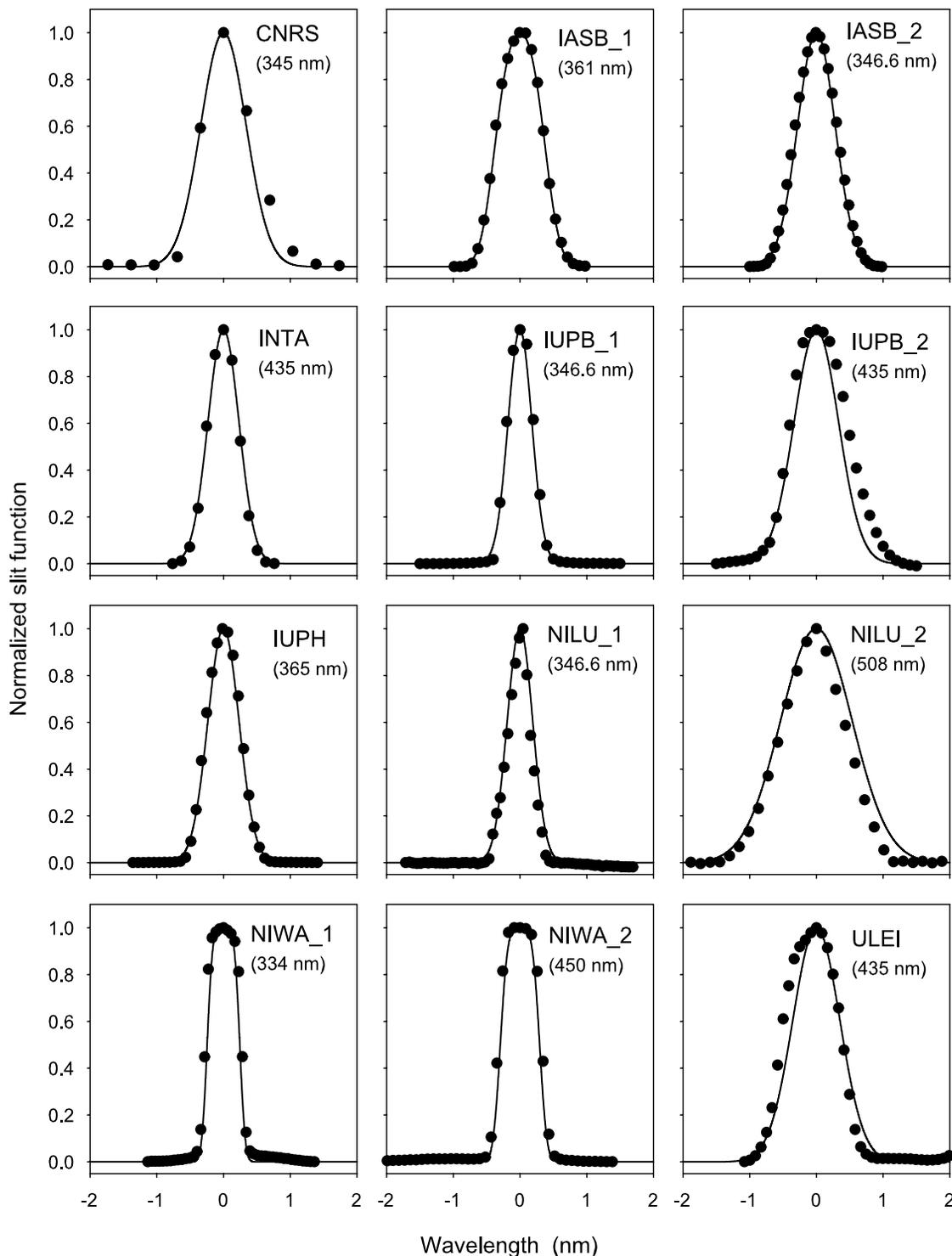
**Figure 3.** Slit functions of all participating instruments. Measured functions using a Hg lamp are represented by dots, while solid lines show the functions derived from zenith sky spectra using the WINDOAS program.
