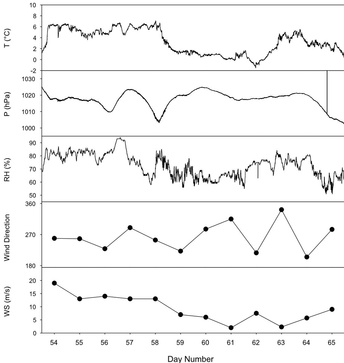
**Figure 1.** Evolution of the meteorological parameters during the NDSC campaign: Temperature, pressure, and relative humidity measured at 15 m elevation at the Andøya Rocket Range facility, and ECMWF wind speed and direction data (at 850 K).
