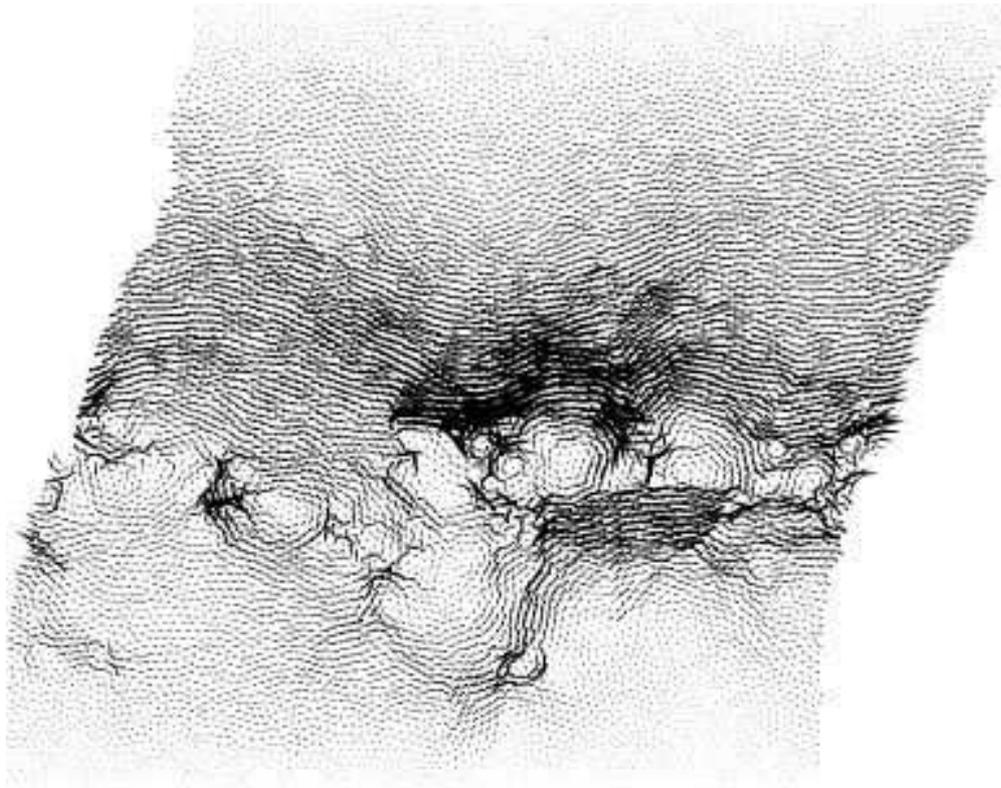
FIG. 7: (Color online) Displacement field associated to an elementary shear band. As it can be seen here, the shear band is due to an alignment of vortices, along the direction of shearing.
