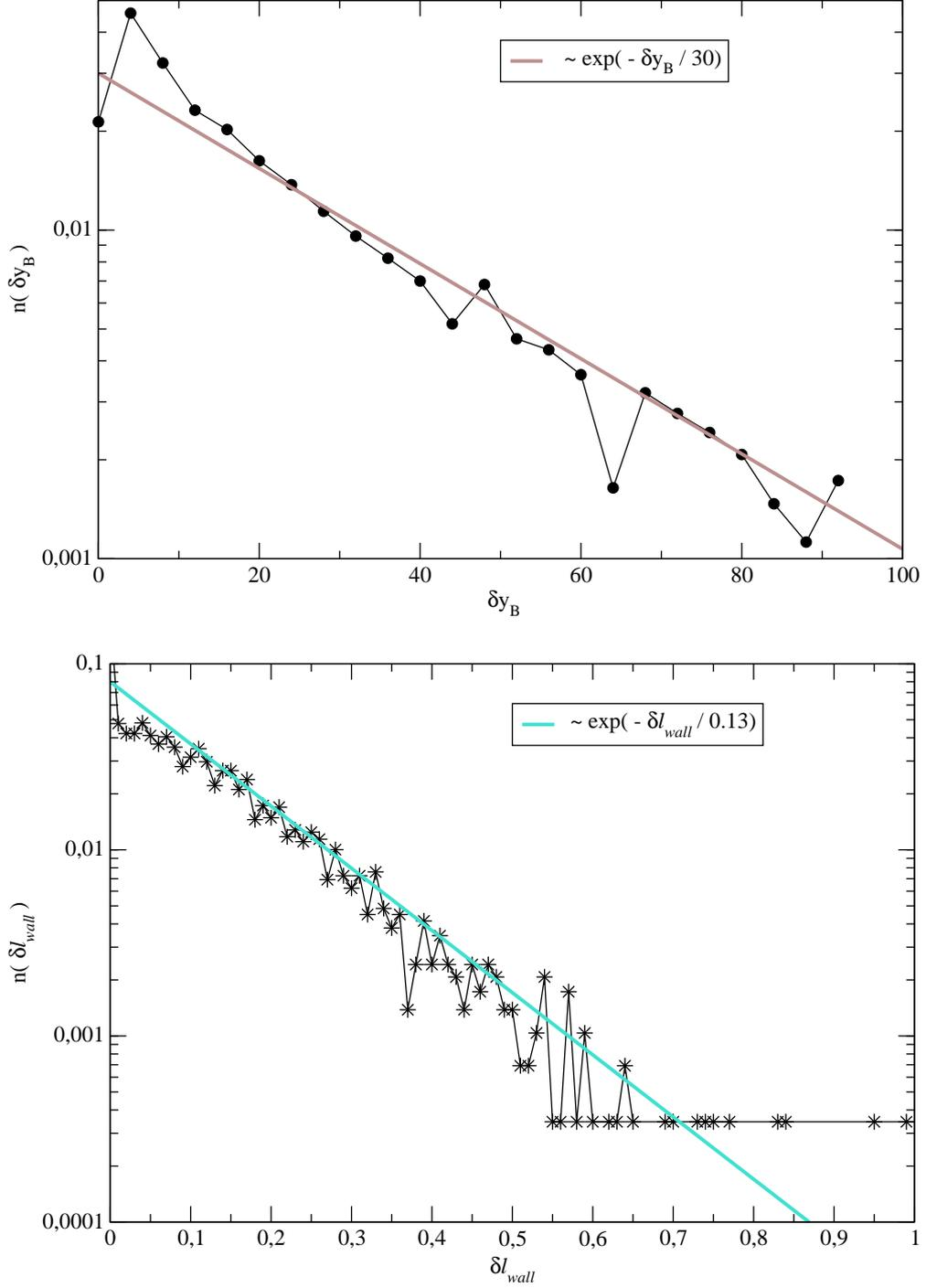
FIG. 10: (Color online) (a) Distribution of the distances  $\delta y_B$  between successive elementary shear bands. The characteristic distance of the exponential fit is  $\xi \approx 30\sigma$ .
