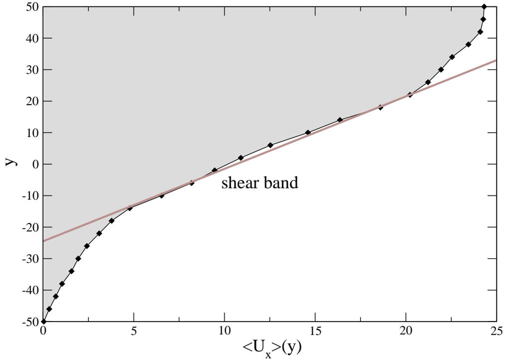
FIG. 3: (Color online) Cumulative displacement in the x-direction (direction of shearing), at various distances  $y$  from the shearing wall, and for a total applied strain  $\epsilon_{xy} \approx 15\%$ . A large shear band appears here in the center.
