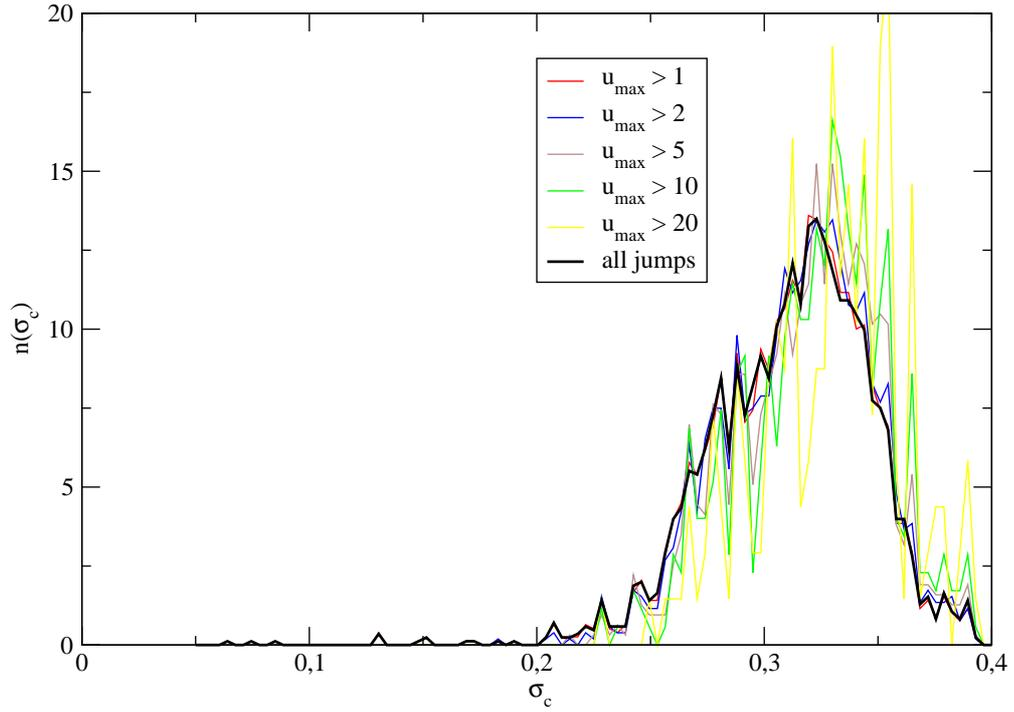
FIG. 9: (Color online) Distribution of plastic thresholds just before a plastic event occurs. This distribution does not depend significantly on the amplitude of the maximum  $u_{\max}$  of the non-affine displacement during the event (contrary to the distribution of the energy drops).
