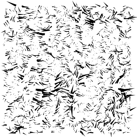
FIG. 1: Inhomogeneous part \delta\mathbf{u}(\mathbf{r}) of the displacement field \mathbf{u}(\mathbf{r}) for the imposed macroscopic uniaxial strain in elongation \epsilon_{xx} = 5.10^{-3} for a silica glass containing N = 42000 particles ( L = 83.8 Å). Projection of the field is done on the (x-z) -plane for all particles with position \mathbf{r} close to the plane, the arrow length being proportional to \delta\mathbf{u}(\mathbf{r}) . The field resides in the linear elastic regime, i.e. has a magnitude varying linearly and reversibly with the applied deformation. As visual inspection shows, it is strongly spatially correlated and involves a substantial fraction of all atoms.
