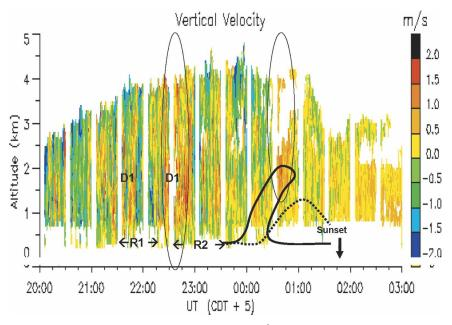
Fig. 8. Time-height plot of the vertical velocity (m s<sup>-1</sup>) observed by the NCAR MAPR/ISS at the IHOP\_2002 profiling site on 22 May 2002. Also shown are the relative locations, in time, of D1, R1, R2, the wind convergence boundaries from GLOW, sunset time, and oval regions of relatively high vertical velocity.
