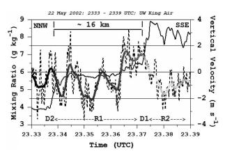
Fig. 5. Water vapor mixing ratio (solid curve) and vertical velocity (dotted curve) data collected by in situ probes aboard the UWKA. A heavily smoothed plot of the vertical velocity data is also shown (thick gray curve). Values shown are for a single leg at 1.6 km AGL as UWKA flew from NNW to SSE across the field of cumulus clouds (its relative location is shown in Fig. 3). Approximate locations of D1, D2, R1, and R2 (refer to Fig. 2) are shown.
