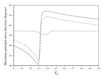
**Figure 11.** Angle between the maximum principal stress and the hinge axis (axis  $\mathbf{e}_1$  in Figure 3) as a function of the normalized position in the hinge  $\tilde{x}_2$ , counted positively in the anticlockwise sense. The entry velocity  $v_i = 10$  mm/yr (solid curve), 6.3 mm/yr (dashed curve), and 1.8 mm/yr (dash-dotted curve). All other parameter values are constant and given in Table 1.
