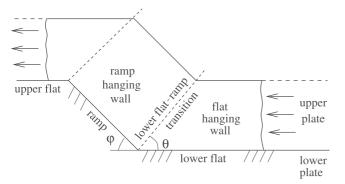
**Figure 1.** Terminology used to describe the geometry of a generic fault-bend fold. The lower flat-ramp transition is called back thrust in frictional materials and hinge in creeping materials.
