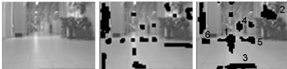
Fig. 3: Input image (left), saliencies extracted by classical processing (center), saliencies extracted by our architecture (right). The numbers on the latter figure specify the temporal order of occurrence.
