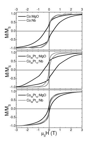
FIG. 2: Normalized hysteresis loops measured at T = 10 K on the samples with Co, Co<sub>85</sub>Pt<sub>15</sub> and Co<sub>58</sub>Pt<sub>42</sub> clusters. The dark lines correspond to the measurements in the MgO matrix and the grey lines correspond to the measurements in the Nb matrix.
