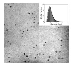
FIG. 1: TEM micrograph of the  $Co_{85}Pt_{15}$  clusters deposited on an amorphous carbon grid. Inset: diameter distribution. The histogram corresponds to the TEM measurements and the continuous line corresponds to a Log-normal fit.
