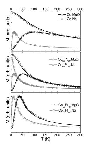
FIG. 3: ZFC-FC curves measured on the Co,  $Co_{85}Pt_{15}$  and  $Co_{58}Pt_{42}$  clusters embedded in MgO and Nb matrices. The curves were recorded in a small field of 5 mT (Co:MgO and  $Co_{85}Pt_{15}$ :MgO) or 10 mT (Co:Nb,  $Co_{85}Pt_{15}$ :Nb,  $Co_{58}Pt_{42}$ :Nb and  $Co_{58}Pt_{42}$ :MgO). The dots correspond to the measurements and the continuous lines correspond to the fits using the model described below.
