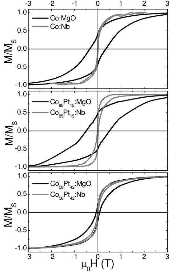
FIG. 2: Normalized hysteresis loops measured at  $T = 10$  K on the samples with Co,  $\text{Co}_{85}\text{Pt}_{15}$  and  $\text{Co}_{58}\text{Pt}_{42}$  clusters. The dark lines correspond to the measurements in the MgO matrix and the grey lines correspond to the measurements in the Nb matrix.
