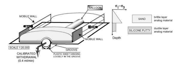
**Figure 14.** Experimental apparatus and the depth-strength profiles used.
