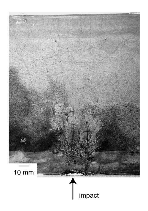
Figure 6: Post-mortem view of an impacted Ductal<sup>®</sup> concrete plate by an aluminum projectile with a confined configuration.
