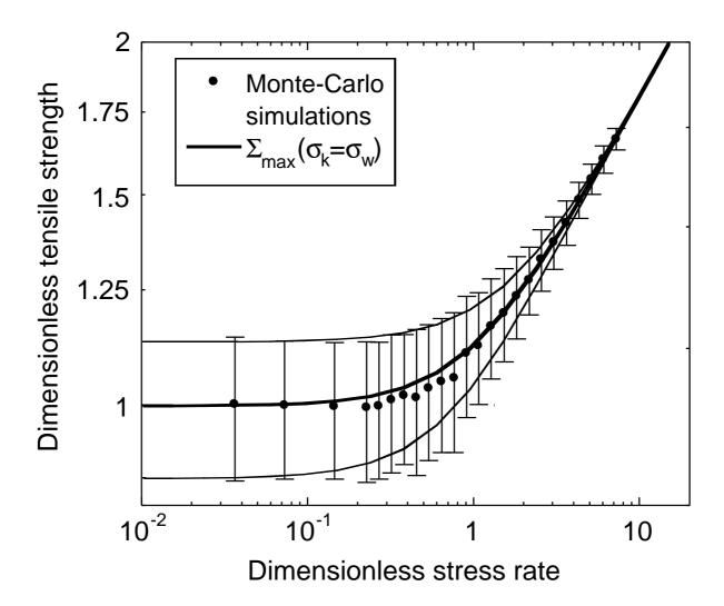
Figure 4: Tensile strength normalized by  $\sigma_w$  vs. stress rate normalized by  $\mathring{\sigma}_t$ . The dots and error bars represent results obtained by Monte-Carlo simulations (500 realizations/point) and their standard deviation when m=9.5 and n=3. The curves are obtained by using Eqn. (26)
