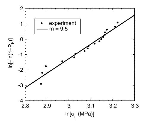
Figure 1: Weibull plot of Ductal® submitted to three-point flexure.
