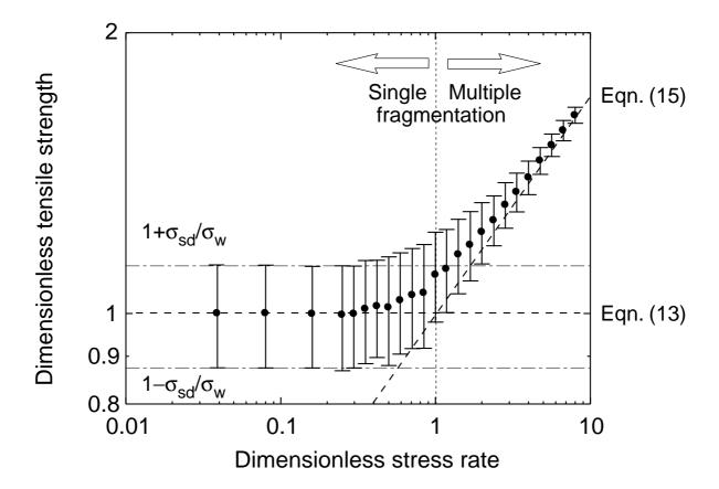
Figure 3: Tensile strength normalized by  $\sigma_w$  vs. stress rate normalized by  $\overset{\bullet}{\sigma}_t$ . The dots and error bars represent results obtained by Monte-Carlo simulations (500 realizations/point) and their standard deviation when m=9.5 and n=3. The curves are obtained by using Eqns. (13) and (15)
