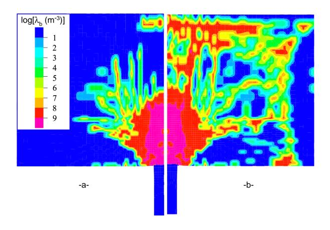
Figure 7: Contour of crack density associated to the first principal direction 35  $\mu$ s (a) and 50  $\mu$ s (b) after impact in a confined EOI experiment on Ductal<sup>®</sup>.
