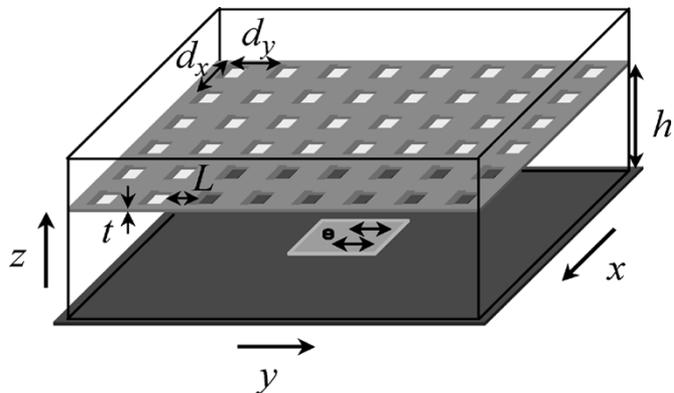
Fig. 1. Schematic representation of the antenna based on a Fabry–Perot cavity, the black lines delimit the volume occupied by the foam. For the prototype  $L = 3.06$  mm,  $t = 0.14$  mm,  $d_x = d_y = 5.8$  mm, and  $h = 9$  mm.
