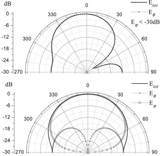
Fig. 4. Radiation patterns (normalized dB scale) of the patch without the grid in the E plane and the H plane. In the E plane, the  $E_\varphi$  component is not visible since it is much less than  $-30$  dB.
