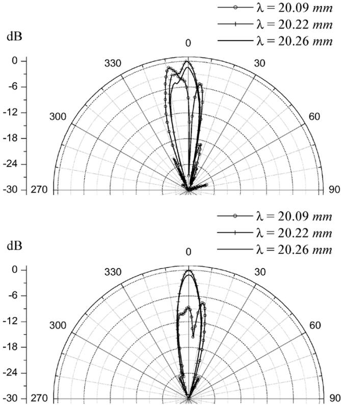
Fig. 8. Experimental radiation patterns (normalized decibels scale) of the antenna in the E plane (top) and the H plane (bottom). The radiation patterns have been normalized with respect to the maximum of emission for the three wavelengths.
