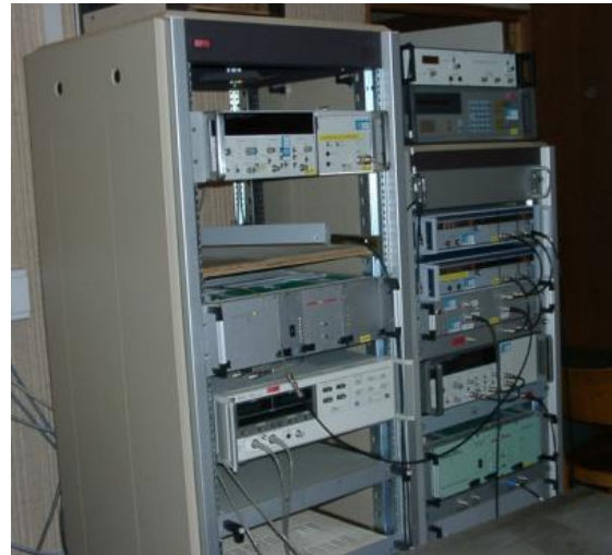
Fig. 2. Frequency stability calibration bench.
