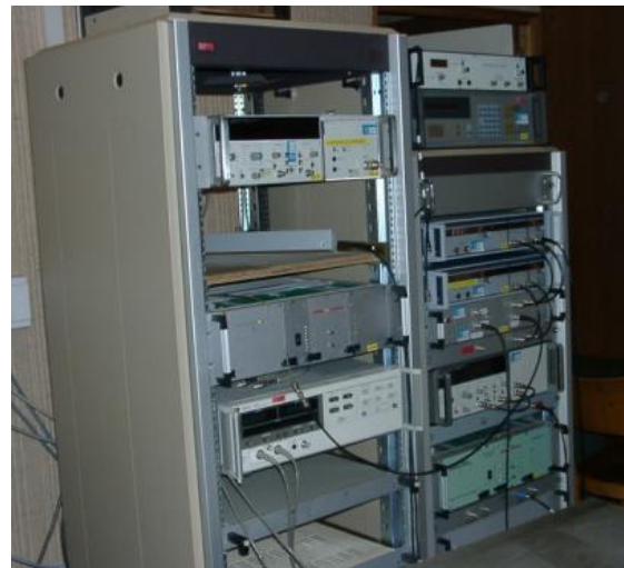
Fig. 2. Frequency stability calibration bench.
