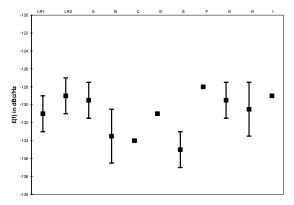
**Figure 4:** SSB phase noise (dBc/Hz) at 100Hz from the 100MHz carrier. Uncertainties given at 2σ
