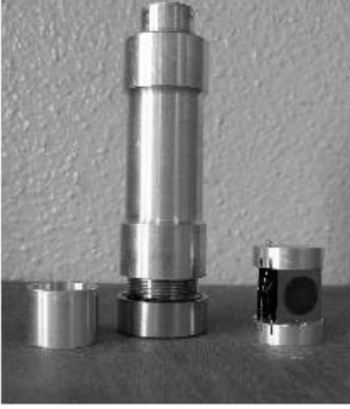
Fig. 2. Photograph of the sample container designed for neutron scattering experiments, in order to control the orientation of the eight aligned porous silicon wafers with respect to the neutron beam.
