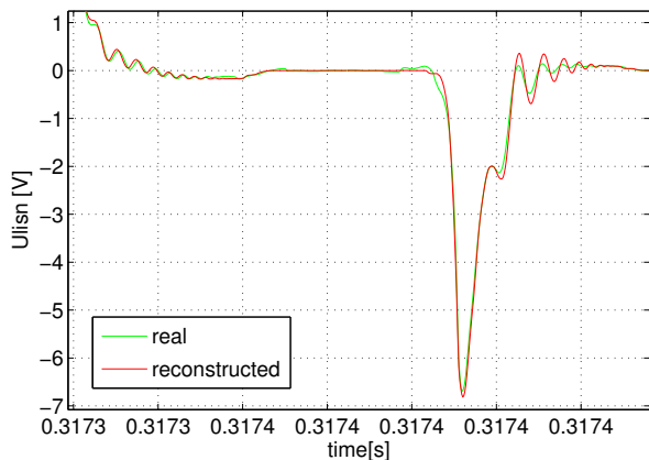
Fig. 8. The measured voltage of semiconductors and LISN waveforms for PWM modulation b) zoom
