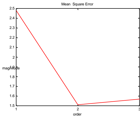
Figure 4 Mean square error for a writing gesture with time delay equal to 100 ms
