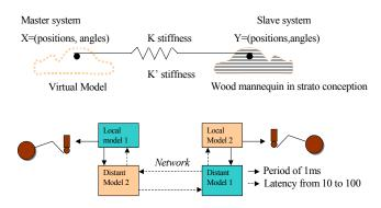
Figure 2. Distant control of the robot in position
