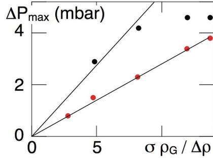
FIG. 2: Position  $\Delta P_{max}$  of the point of maximal slope in the adsorption branch versus the temperature dependent ratio  $\sigma\rho_V/(\rho_L - \rho_V)$ . The straight lines correspond to pore diameters (see text) of 18 and 36 nm.
