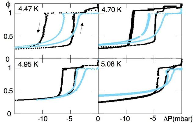
FIG. 1: (a) Isotherms at four temperatures, 4.47, 4.71, 4.96 and 5.08 K, for two aerogels of porosity 95%, B100 (black) and N102 (grey). The liquid fraction  $\Phi$  in aerogel is plotted versus  $\Delta P = P - P_{sat}$ ; for B100, there is a clear change of shape with temperature.
