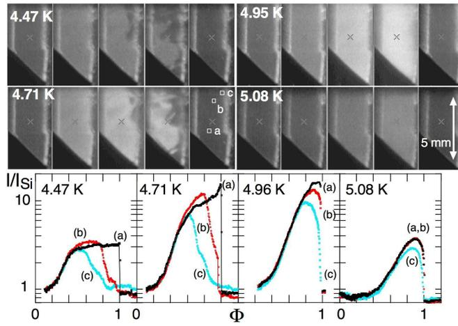
FIG. 3: Images of B100 observed at  $45^\circ$  from the incident laser sheet for helium fractions of 0.1,0.5,0.7,0.9, and 1.0. The curves give the scattered intensity, referred to the empty aerogel situation, for the three regions labelled (a), (b), (c).
