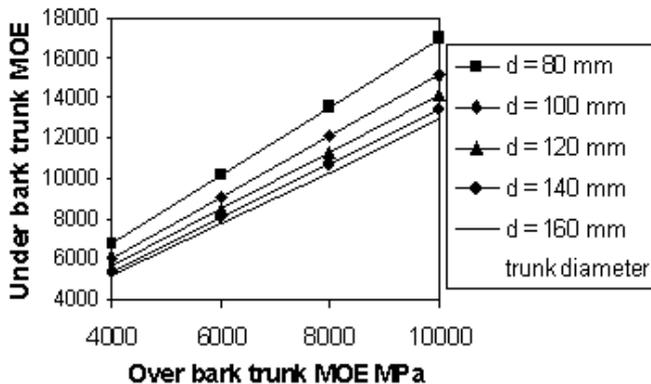
Figure 4. Comparison of the trunk MOE with and without bark.
