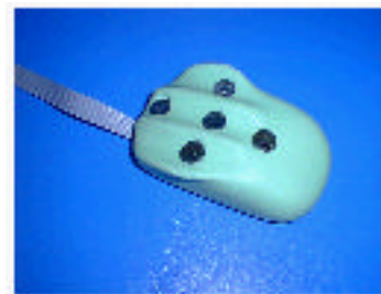
Figure 2: The 'Tactile mouse' including an array of five stimulators
