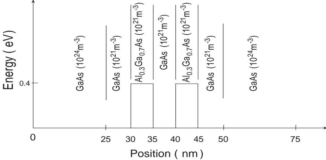
Fig. 1. The double barrier resonant tunneling structure.
