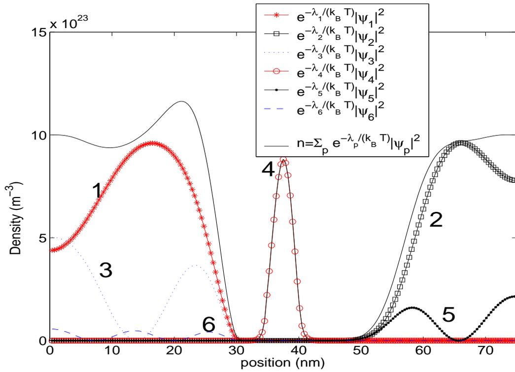
Fig. 8. Density at the peak (Applied bias: 0.25V).
