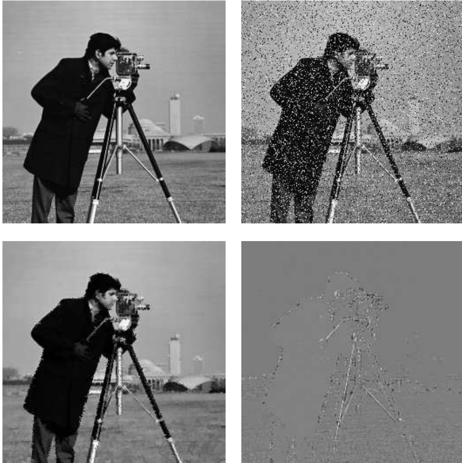
Figure 5: From left to right, top to bottom: (a) the original cameraman image u (size 256 \times 256 ); (b) degraded image v , with impulse noise probability parameter p = 0.2 ; (c) filtered image \tilde{v} , obtained with \varepsilon = 10^{-3} ; (d) image of the difference u - \tilde{v} . It shows that most of the noise has been removed, except at the boundaries of the objects and also in the grass texture.
