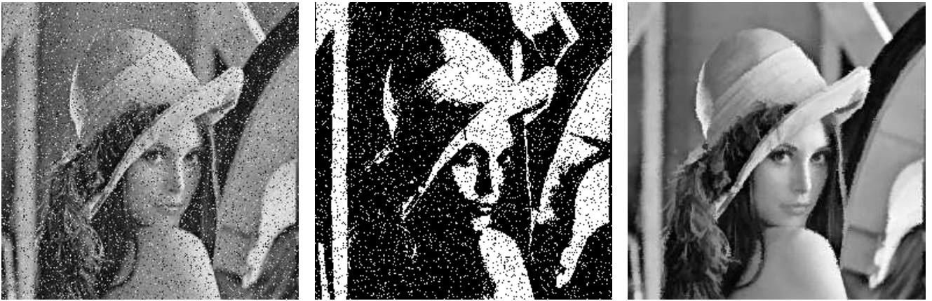
Figure 4: Left: image v obtained with impulse noise with probability parameter p = 0.15 on the Lena image. Middle: thresholded image v_\lambda for the grey level \lambda = 150 . Right: denoised image \tilde{v} obtained by the noise-adapted grain filter T with \varepsilon = 10^{-3} .
