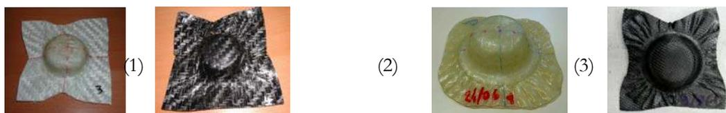
FIG. 6 – (1) Twintex (PP/Verre)  $T_{Form} \approx 160\sim 190^{\circ} C$  (2) Hexform (Epoxy/Verre)  $T_{Form} \approx 150\sim 180^{\circ} C$
