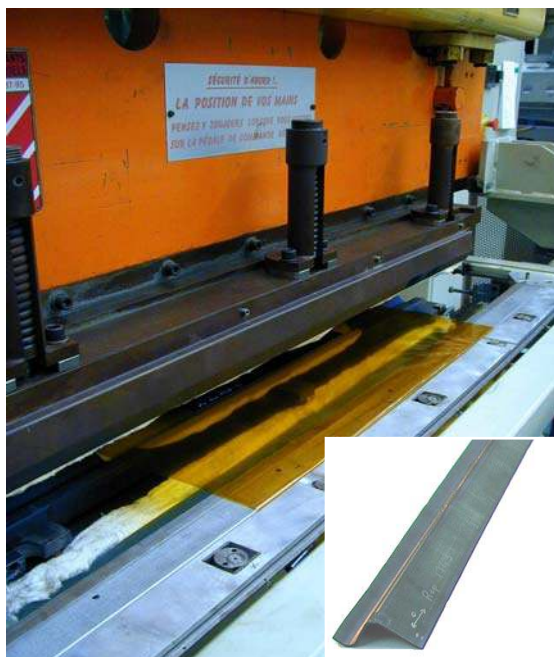
Figure 5. Punch and die (and final shape)
