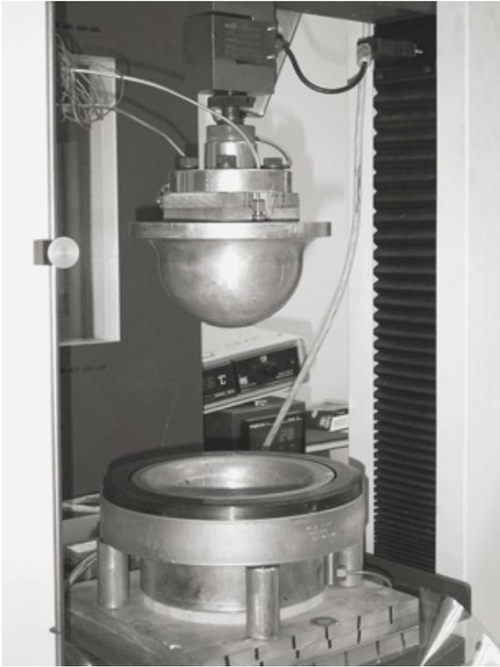
**Figure 1.** *Couple poinçon-matrice*
