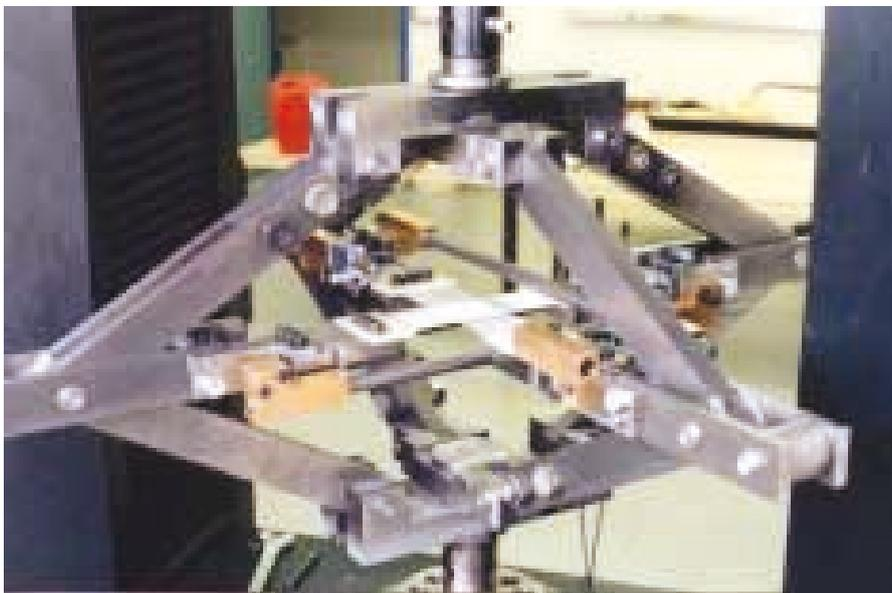
**Figure 7.** *Biaxial tension device*
