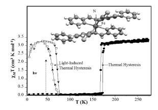
FIG. 1. Temperature dependence of the magnetic susceptibility times the temperature  $\chi_{\rm M}T$  on cooling and heating modes for the  $[{\rm Fe}({\rm PM\text{-}BiA})_2({\rm NCS})_2]$  compound represented here. The first-order transition occurs around 170 K with a thermal hysteresis of 5 K. Under continuous laser irradiation (5 mW/cm² at 830 nm) the HS state can be photoinduced (arrow) and a quasistatic light-induced thermal hysteresis (LITH) appears between the cooling and warming modes.
