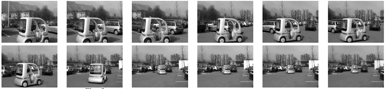
Fig. 5: Experimental results: Sequence showing an avoidance manoeuvre.
