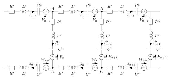
Figure 2: A section of the birdcage equivalent circuit
