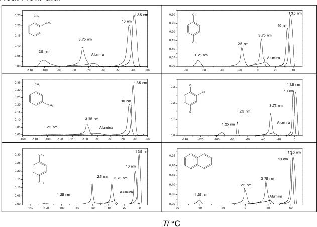
**Figure 2**: Thermograms of the six organic compounds (*o, m, p*-xylene, *p*-dichlorobenzene, *1,2,4*-trichlorobenzene and naphthalene) soaking the silica gel samples referenced 13.5, 10, 3.75, 2.5 and 1.25 nm (see table 1). The thermograms of the six solvents confined inside the alumina test sample are also presented. Only the peaks of confined solvent are shown. The decreasing temperature rate is 0.7 °C.min
