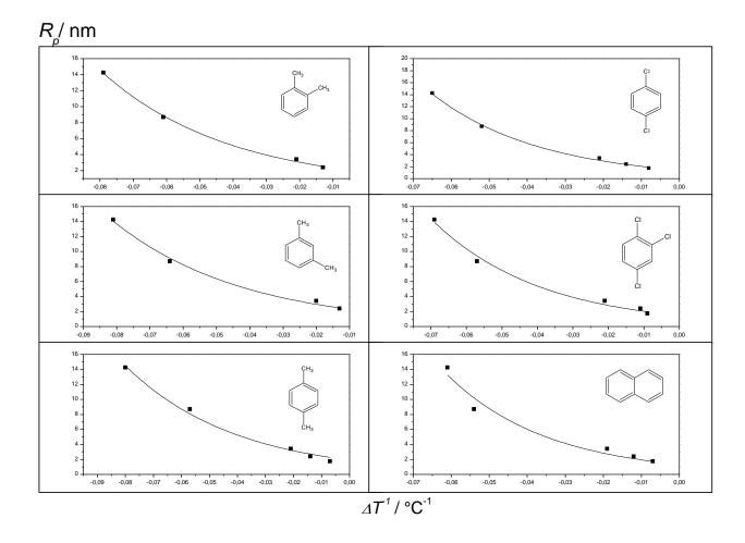
**Figure 3**: Pore radii  $(R_p)$  of the silica gel calibration samples  $vs(\Delta T^l)$  for each of the six solvents (o, m, p-xylene, p-dichlorobenzene, 1,2,4-trichlorobenzene and naphthalene).
