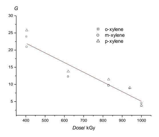
**Figure 9**: Evolution of the degree of swelling G for the three xylene isomers as a function of the irradiation dose received by the polymer. The line corresponding to a linear evolution is drawn as guide for the eye.
