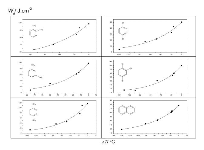
**Figure 4**: Plots of apparent energy  $(W_a)$  of crystallization vs freezing temperature depression  $(\Delta T)$  of the confined solvents. This change in the thermal transition energy takes into account two contributions: the first is the decreasing of latent enthalpy when the temperature decreases and the second is the fact of an amount of the confined solvent remains adsorbed on the wall of the divided medium and does not take part to the thermal transition.
