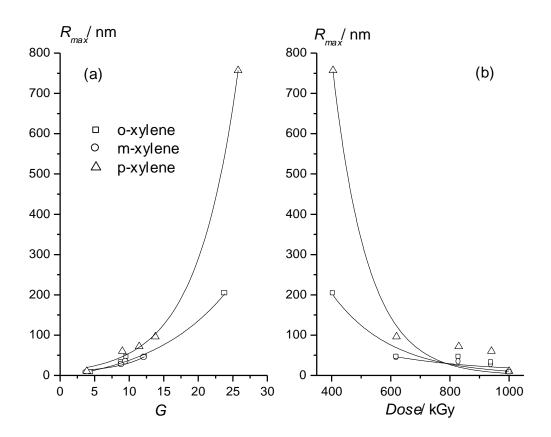
**Figure 8**: Evolution of the maximum of the Mesh Size Distribution  $(R_{max})$  for the different polyolefins as a function of the swelling ratio (a) and the irradiation dose (b) for the three xylene isomers. Lines are drawn as a guide for the eye.
