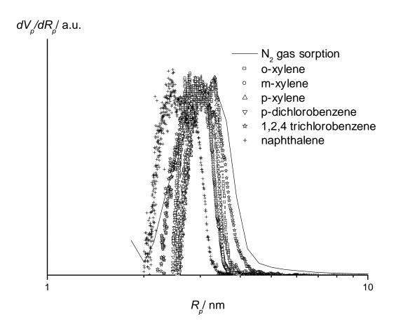
**Figure 5**: Pore size distributions of the alumina test sample calculated from the  $N_2$  sorption technique (line) compared with that derived from thermoporosimetry calculation (symbols) using each of the six solvents (o,  $m_1$ , $p_2$ -xylene,  $p_2$ -dichlorobenzene, 1,2,4-trichlorobenzene and naphthalene) as condensate.
