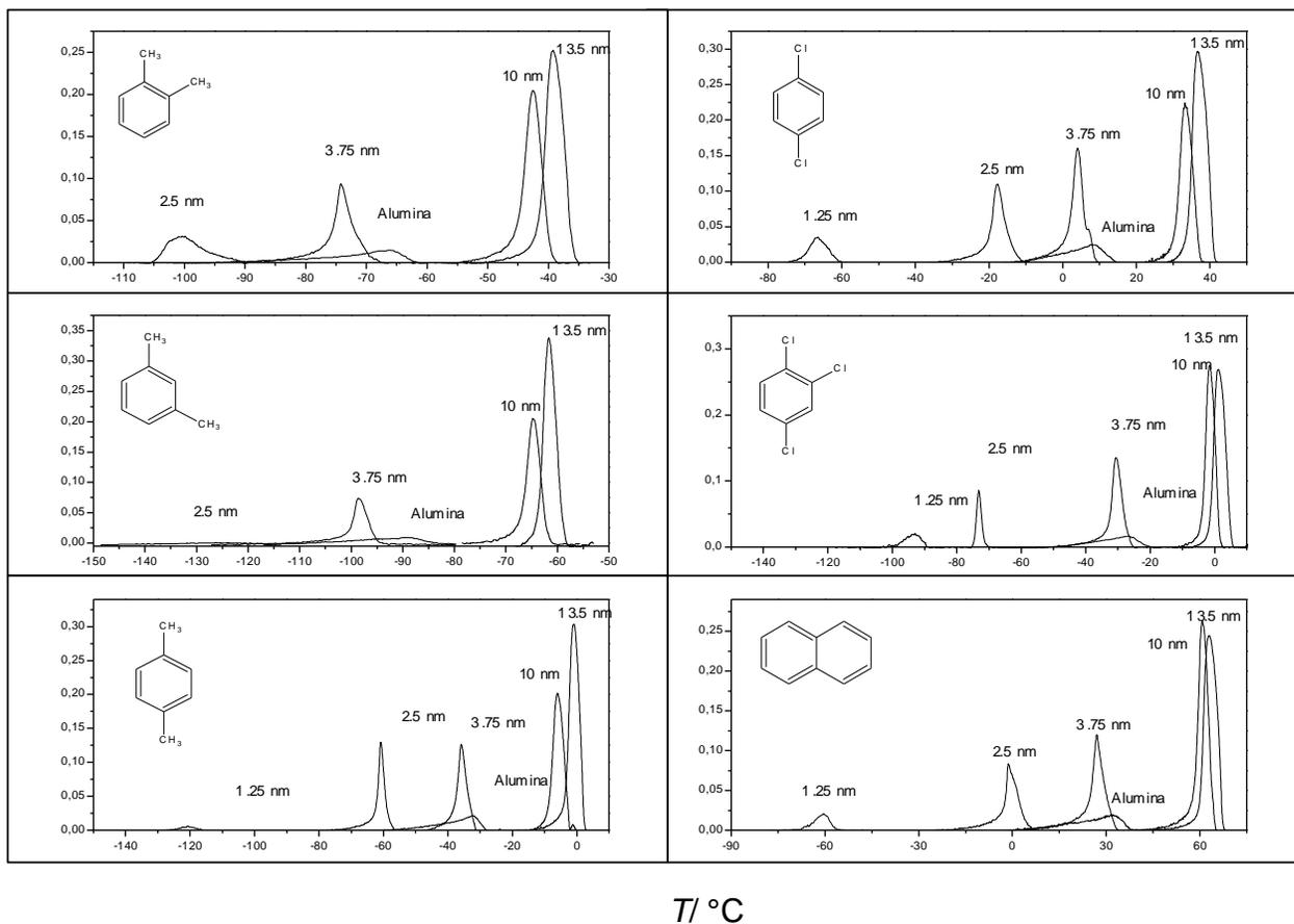
**Figure 2:** Thermograms of the six organic compounds (*o*, *m*, *p*-xylene, *p*-dichlorobenzene, 1,2,4-trichlorobenzene and naphthalene) soaking the silica gel samples referenced 13.5, 10, 3.75, 2.5 and 1.25 nm (see table 1). The thermograms of the six solvents confined inside the alumina test sample are also presented. Only the peaks of confined solvent are shown. The decreasing temperature rate is  $0.7^{\circ}\text{C}\cdot\text{min}^{-1}$ .
