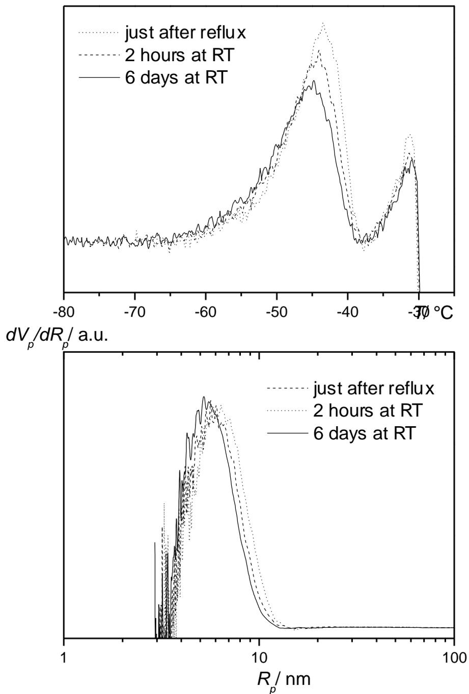
**Figure 6:** Thermograms (a) and mesh size distributions (MSD) (b) of cross-linked polyethylene sample having received a dose of 1000 kGy and swollen with *o*-xylene. The sample is analyzed, just after the reflux was stopped (dotted line), after two hour resting at room temperature (dashed line) and after six days at room temperature (solid line).
