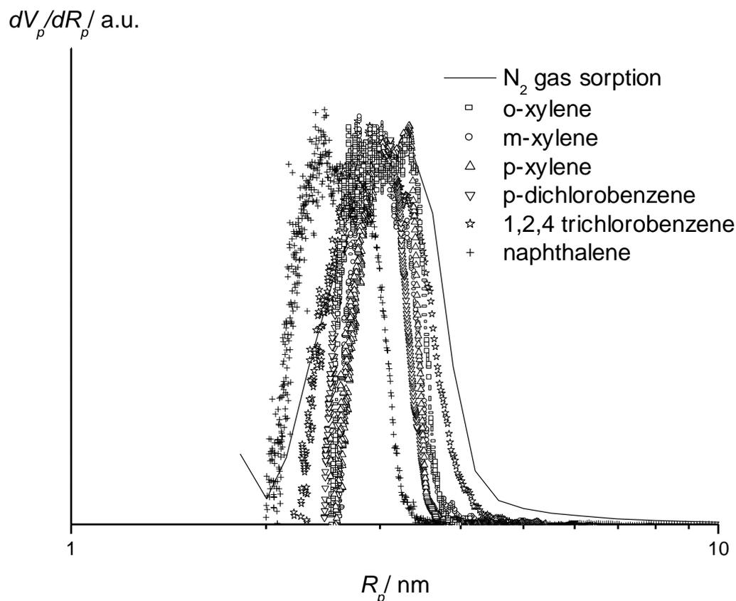
**Figure 5:** Pore size distributions of the alumina test sample calculated from the  $N_2$  sorption technique (line) compared with that derived from thermoporosimetry calculation (symbols) using each of the six solvents (*o*, *m*, *p*-xylene, *p*-dichlorobenzene, *1,2,4*-trichlorobenzene and naphthalene) as condensate.
