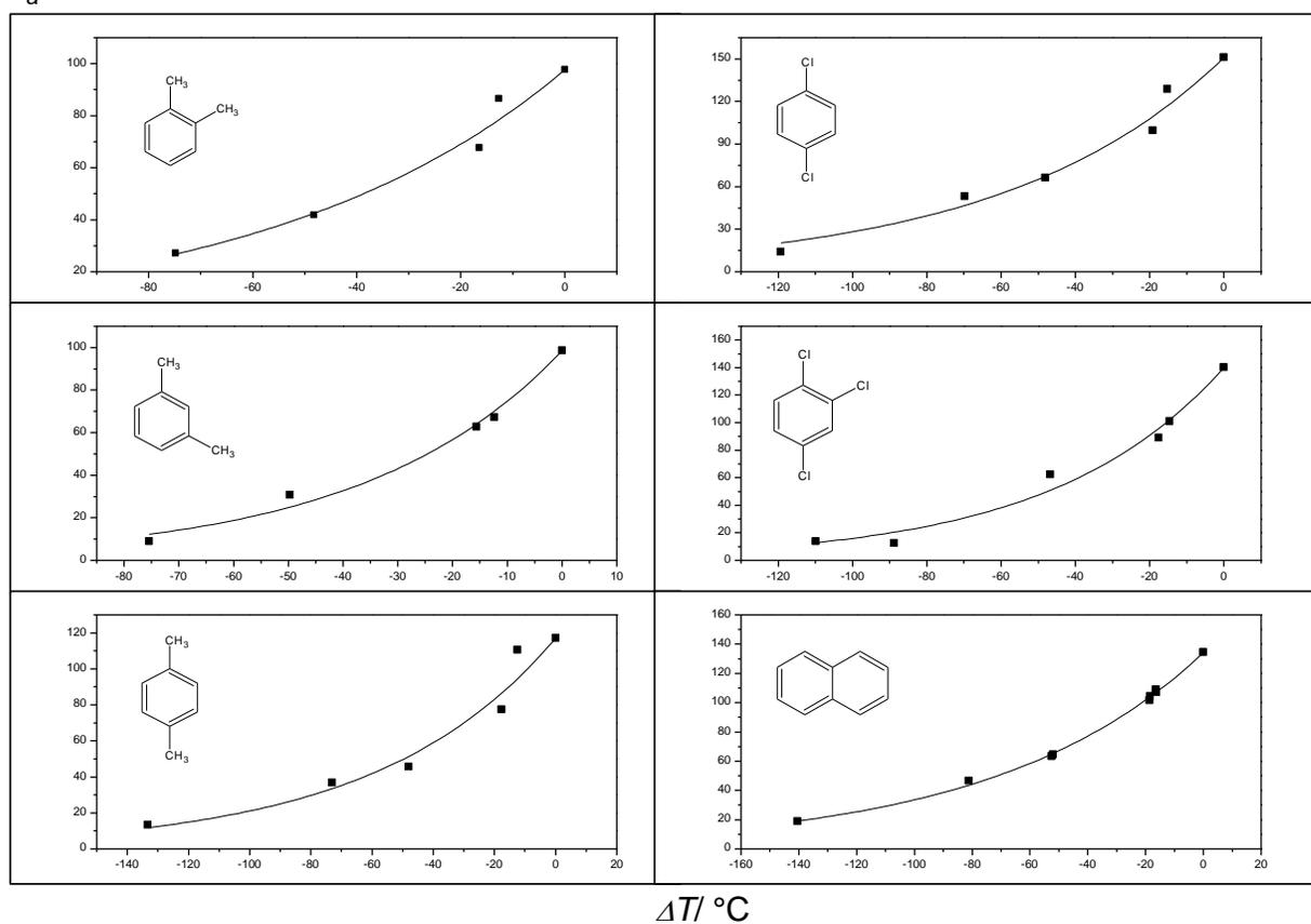
**Figure 4:** Plots of apparent energy ( $W_a$ ) of crystallization vs freezing temperature depression ( $\Delta T$ ) of the confined solvents. This change in the thermal transition energy takes into account two contributions: the first is the decreasing of latent enthalpy when the temperature decreases and the second is the fact of an amount of the confined solvent remains adsorbed on the wall of the divided medium and does not take part to the thermal transition.
