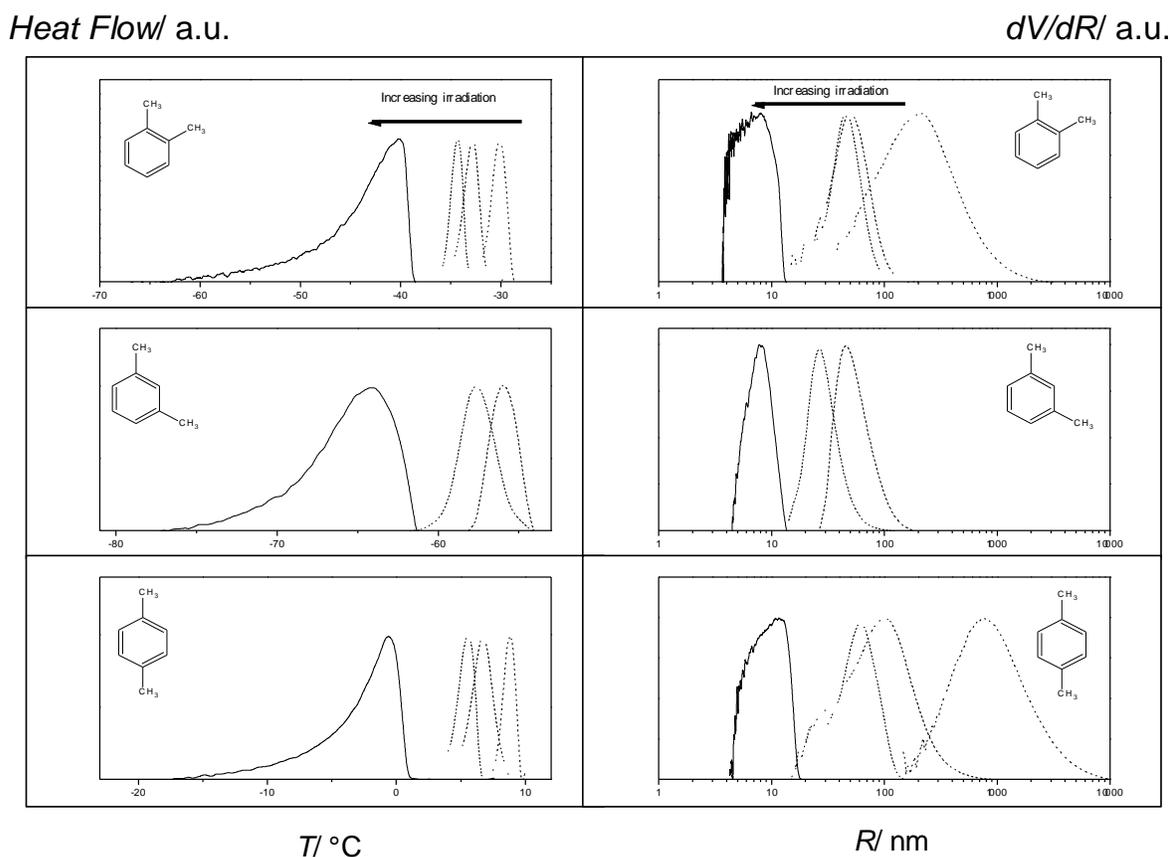
**Figure 7:** Thermograms (on the left) and corresponding mesh size distributions (on the right) of PE1000kGy (solid line), PP940kGy (dotted line), PP830kGy (dashed line), PP620kGy (dash dotted line)
