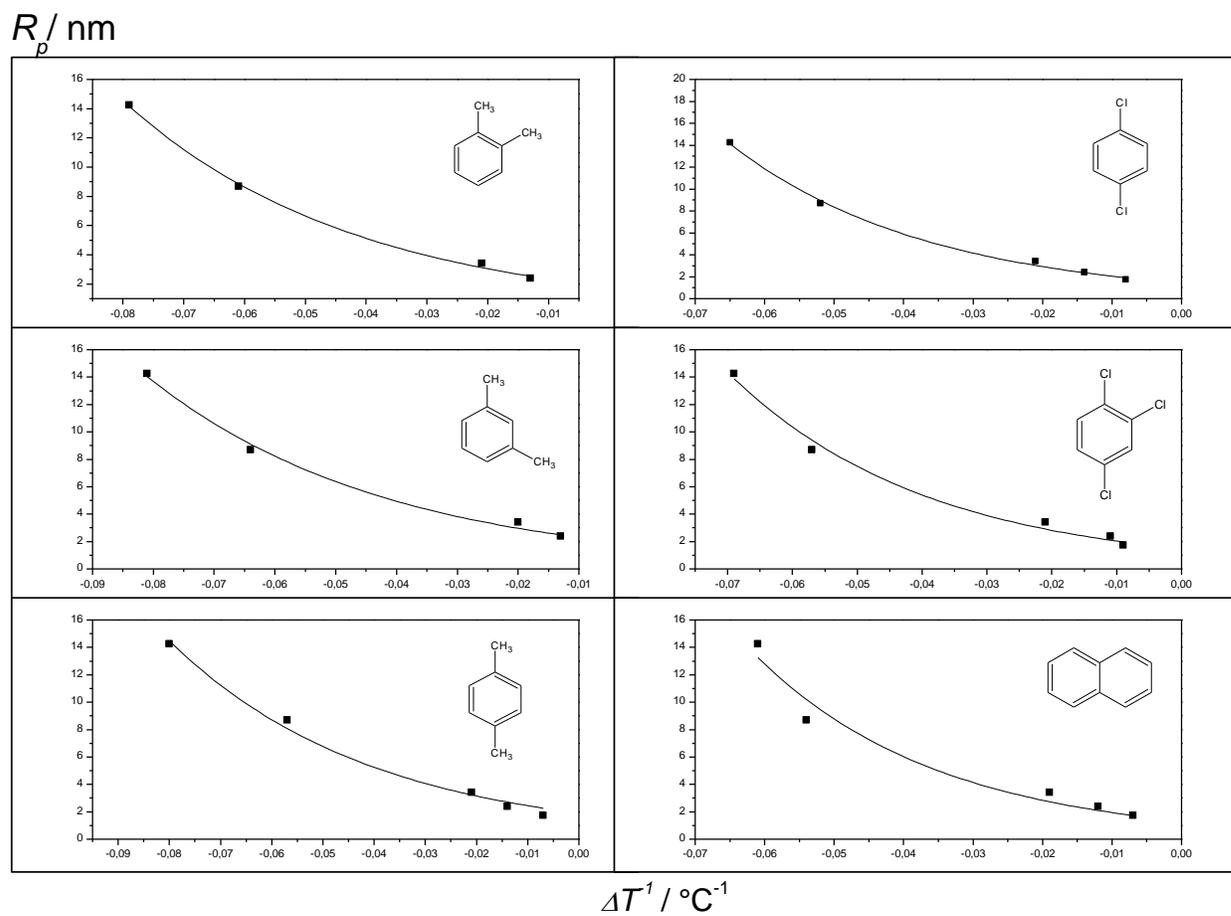
**Figure 3:** Pore radii ( $R_p$ ) of the silica gel calibration samples vs ( $\Delta T^{-1}$ ) for each of the six solvents (o, m, p-xylene, p-dichlorobenzene, 1,2,4-trichlorobenzene and naphthalene).
